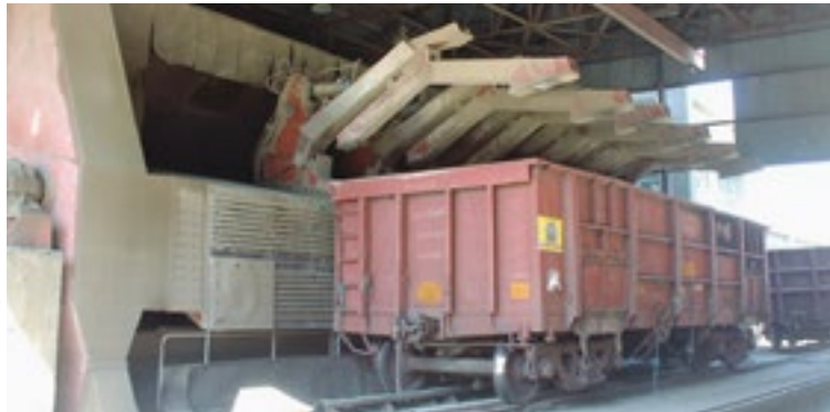
Hydraulically operated wagon tippler of unloading capacity 20 wagons per hour for Clinker & Gypsum rakes unloading at Sonar Bangla Cement (Grinding Unit)
