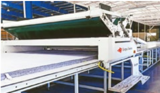
Spreading Machine with cutting Facility for Bedlinen
